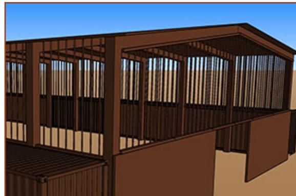
From there we would use thin walled tubing, metal tubing, and weld the thin walled tubing going up vertically, so we have bars. So the first half is a solid wall with the cargo containers, then barring all the way around the top half of the flight chamber so that there would be lots of ventilation and the birds could see out.
